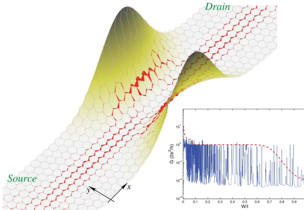
FIG. 4. (Color online) A direct demonstration of Klein tunneling in graphene QPC: three-dimensional view of current flow with respect to the potential profile of the QPC. The sizes of the arrows indicate the values of the current flow. The Fermi energy is  $E_F = 0.8$ . Inset: solid line is the fractal-like conductance fluctuations of the graphene QPC as a result of Klein tunneling; dashed line is the smooth conductance variation in the corresponding nonrelativistic QPC.
