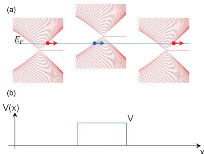
FIG. 2. (Color online) (a) Illustration of Klein tunneling of graphene quasiparticles. (b) Simplified potential profile, a square potential barrier of height  $V$  along the direction of the ribbon.
