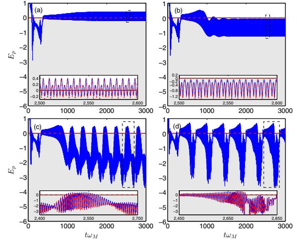
FIG. 3 (color online). (a)–(d) Time evolution of  $E_p$  for four values of the laser driving power  $\tilde{P}$  as specified by the vertical red dotted lines in Fig. 2(a). Insets show the respective zoom-in regions indicated by the black dashed boxes, and the thin red dashed lines represent the results from the ensemble approach. The shaded regions correspond to nonphysical results and  $E_N = \max[0, E_p]$ .
