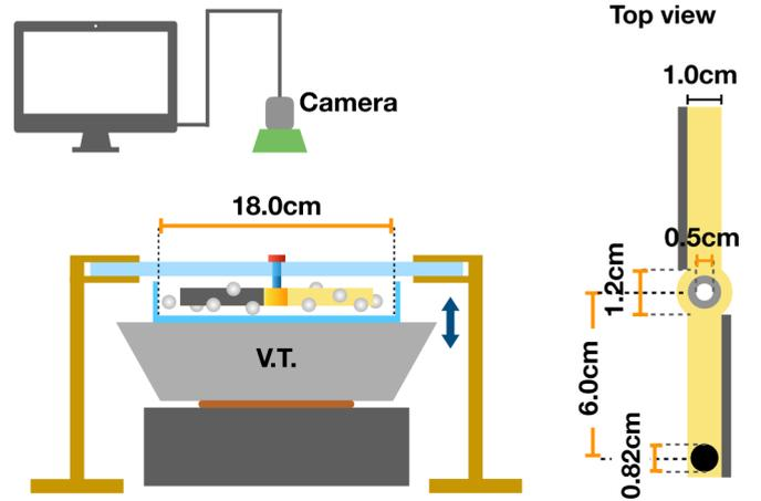
FIG. 1. The experimental setup. The Brownian motor with a circular tracking mark (the black point on the motor) is fixed on the floating cover. The vibration table (V.T.) supplies vertical sinusoidal vibration and maintains the steady granular gas state. The vibration amplitude is 0.15 mm, and the frequency is 100 Hz. The distance between the center of the motor and the center of the mark point is  $l_m = 6.0$  cm, and the diameter of the container is  $d = 18.0$  cm.
