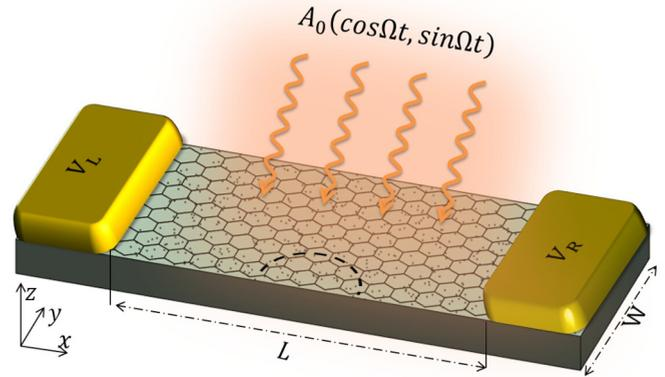
FIG. 1. Schematic illustration of the system configuration. A two-terminal graphene nanoribbon of length  $L$  and width  $W$  is irradiated by a circularly polarized light beam of strength  $A_0$  and frequency  $\Omega$ . The random black dots denote the on-site potential disorder. The left and right leads are shielded from light irradiation by the electrodes. The quantities  $V_{L,R}$  represent the potential at the left and right leads, respectively.
