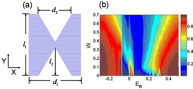
FIG. 4. (Color online) (a) Schematic illustration of a wedge-shaped graphene junction. The device parameters are  $l_1=89a_0$ ,  $l_2=41a_0$ ,  $d_1=42.5a$ , and  $d_2=27a$ . (b) Contour plot of  $G$  in the  $(W, E_R)$  plane for  $E_L=-0.1$  and  $\phi=0$ .
